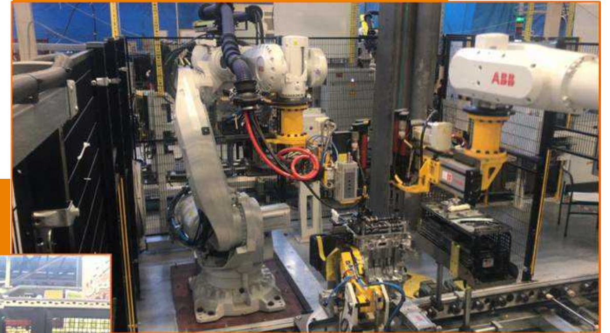
Robotic Tightening Process
